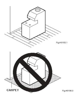
**NOTE**: The heater should be located in an area where water leakage will not result in damage to the area adjacent to the appliance or to the structure. When such locations cannot be avoided, it is recommended that a suitable drain pan, adequately drained, be installed under the appliance. The pan must not restrict air flow.
